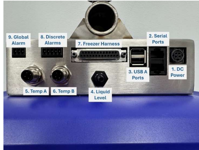
Figure 79. Temperature Sensor, Liquid Level, Freezer Harness and DC Power Connections
