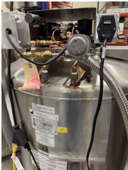
Figure 80: AC Power Cord Connection to Freezer Power Entry Module
