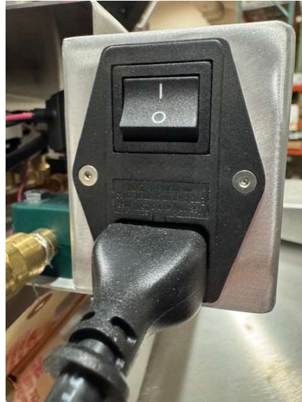
Figure 80: AC Power Cord Connection to Freezer Power Entry Module
