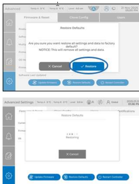
Figure 50. Restore To Defaults
