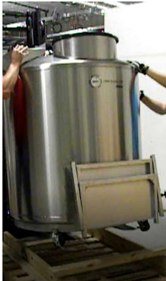
Figure 77. Removal of Pallet from Underneath Freezer
