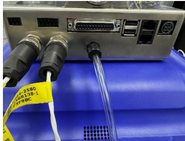
Figure 5. Pressure Tube Connect to CryoVerse Connect
