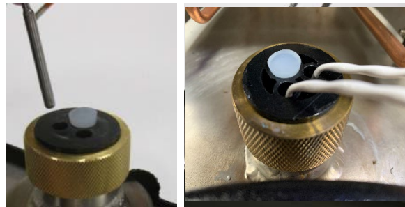
Figure 3. Temperature Sensor Tube Assembly
