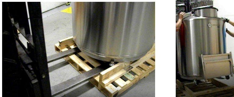
Figure 2: Removal of Freezer From Skid with Forklift
