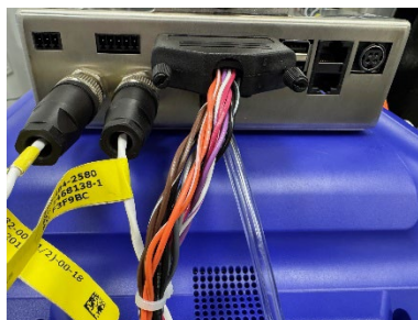
Figure 6. Freezer Harness Connection to CryoVerse Connect DB-25
