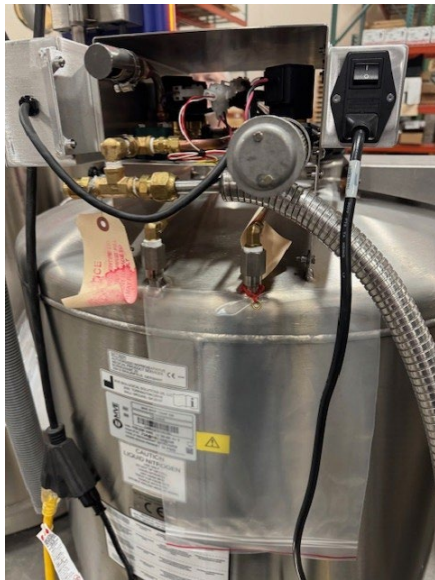
Figure 89: AC Power Cord Connection to Freezer Power Entry Module
