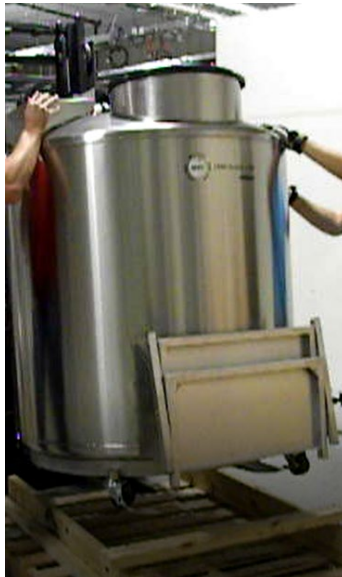
Figure 86. Removal of Pallet from Underneath Freezer
