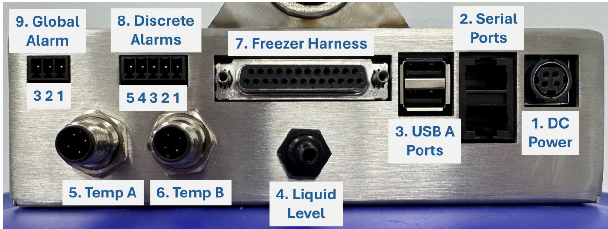
Figure 81. CryoVerse Connect Global and Discrete Alarm Pin-outs
