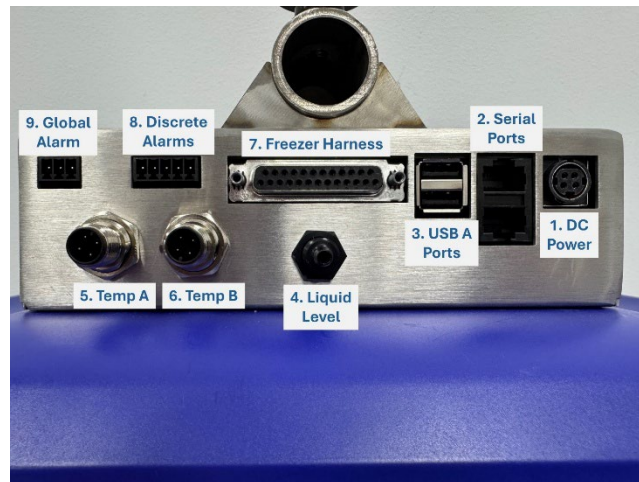
Figure 90: DC Power Supply Connection
