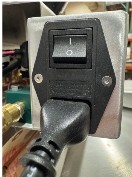
Figure 89: AC Power Cord Connection to Freezer Power Entry Module
