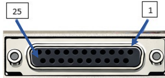
Figure 80. Pin 1 and 25 Locations
