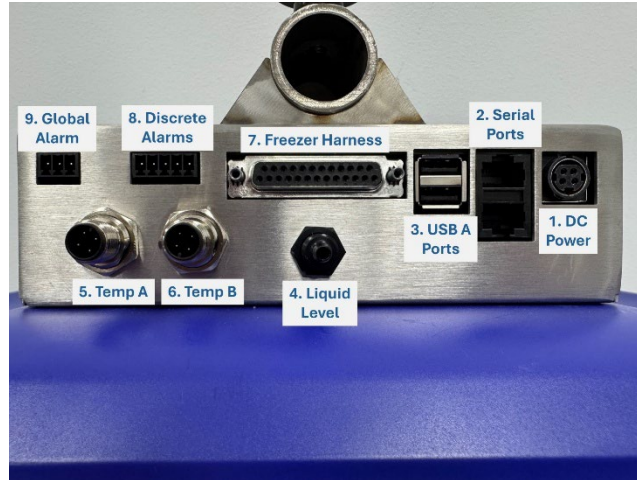
Figure 88. Temperature Sensor, Liquid Level, Freezer Harness and DC Power Connections
