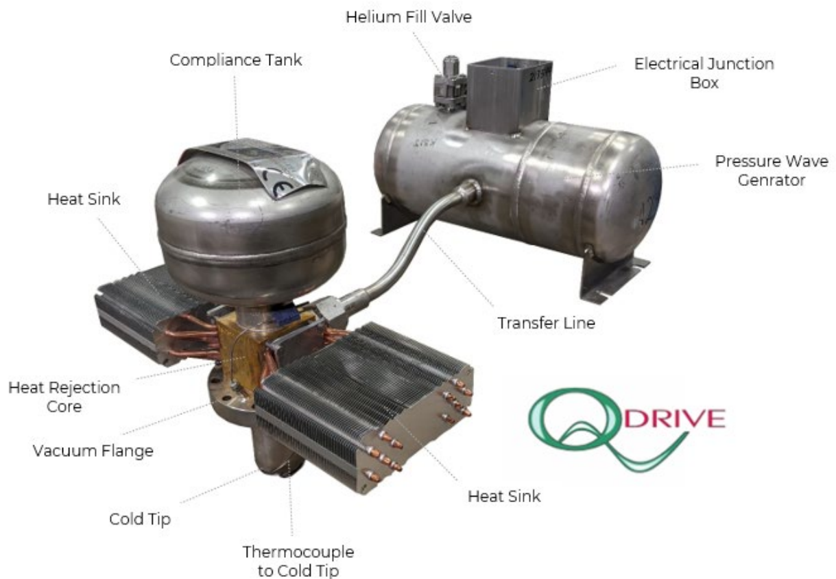
Figure 4: QDRIVE Cryocooler System
