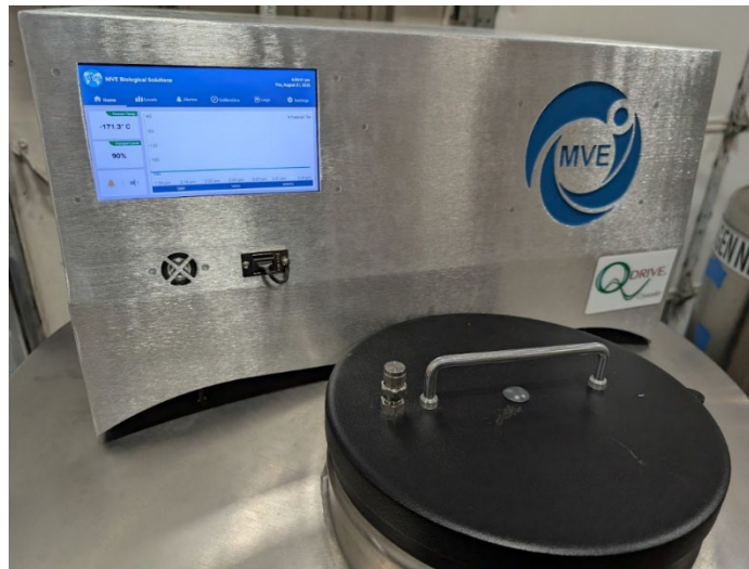
Figure 14: Freezer Lid proximity switch location
