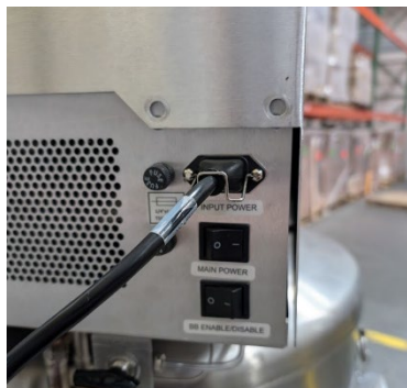
Figure 21: Power cord connected to Fusion® input power receptacle
