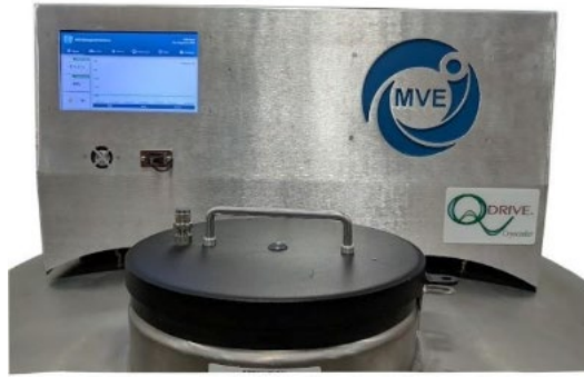
Figure 8: Freezer Lid Installed (Correct Orientation)
