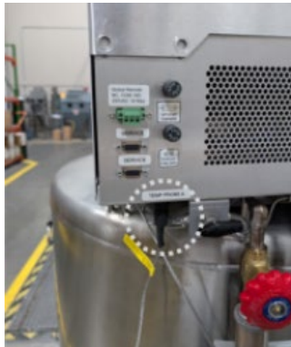
Figure 11: RTD connected to the Liquefier shroud
