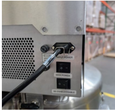
Figure 19: Power cord connected to Fusion® input power receptacle
