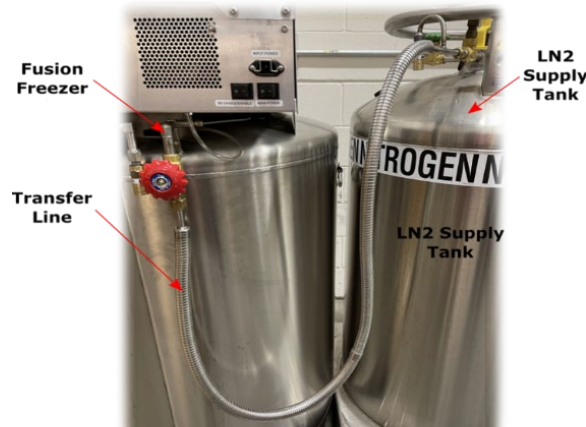
Figure 22: Transfer hose connection
