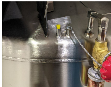
Figure 12: Temperature sensor ports with yellow plug for aftermarket sensor
