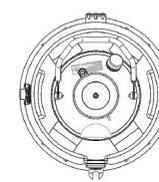
Shock absorbing foam in the PPSC helps prevent damage to the dewar. Illustration shows top view of the tank in the PPSC.
