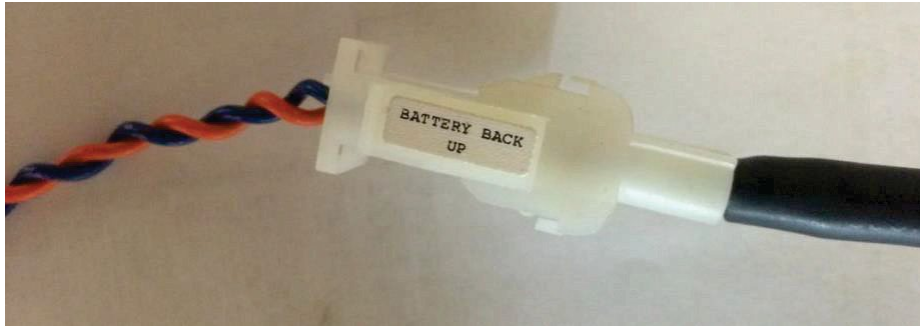
Battery Backup Connector. [Black – From the Battery Backup. Dark Blue/Orange – From the MVE TS Wiring Harness]
