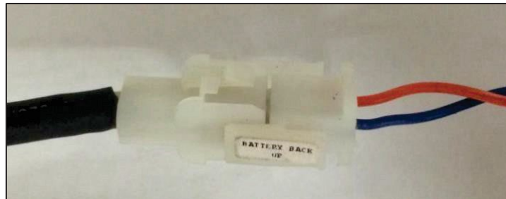
Battery Backup Connector. [Black – From the Battery Backup. Dark Blue/Orange – From the MVE TS Wiring Harness]
