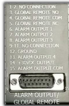
Figure 7: MVE TS remote alarm contacts
