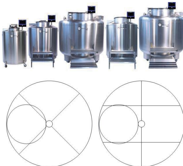
Figure 1: Top-view of HE Freezer showing offset neck and P and R turn-trays
