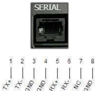
Figure 10: MVE TS serial port and RS-485 4-wire pin diagram
