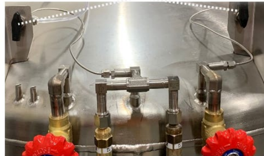
Figure 25: Isolation valve: Both valves in the open, horizontal position (left), both valves in the closed, vertical position (right)
