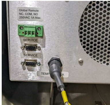
Figure 12: RTD connected to the Liquefier shroud
