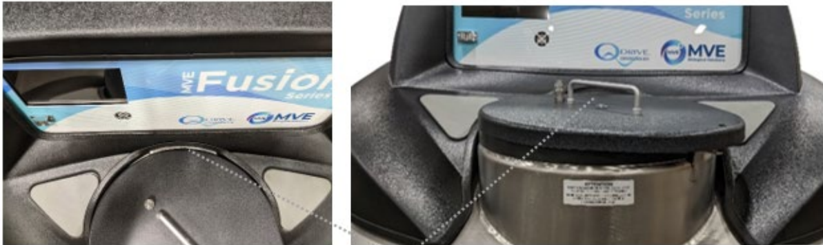
Proximity Switch Location
