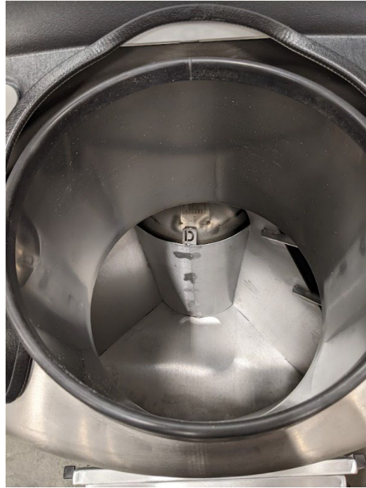
Figure 15: View inside Fusion 1526 Sample storage area with inventory systems
