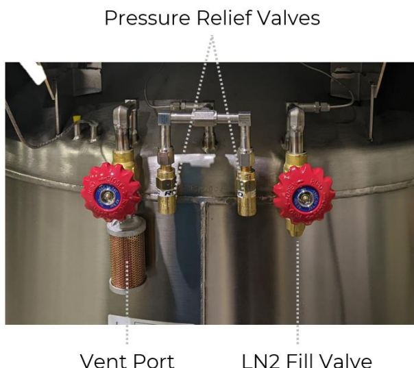
Figure 24: Vent port, dual Pressure relief valves, LN 2 fill valve
