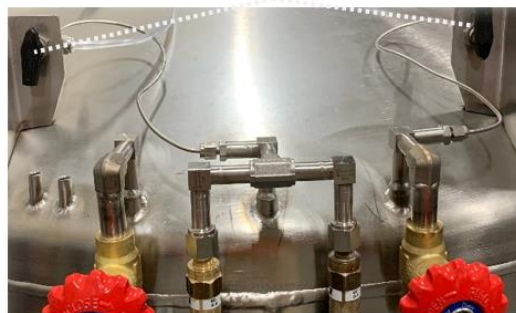
Figure 28: Isolation valve: Both valves in the open, horizontal position (left), both valves in the closed, vertical position (right)
