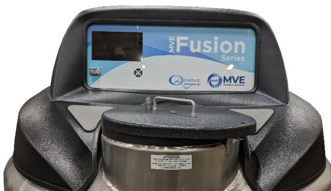
Figure 8: Freezer Lid Installed (Correct Orientation)
