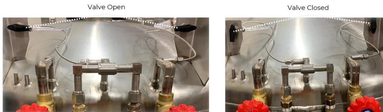
Figure 18: Isolation valve: Both valves in the open, horizontal position (left), both valves in the closed, vertical position (right)
