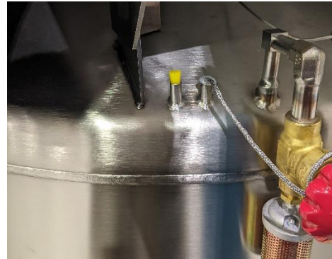
Figure 13: Temperature sensor ports with yellow plug for aftermarket sensor
