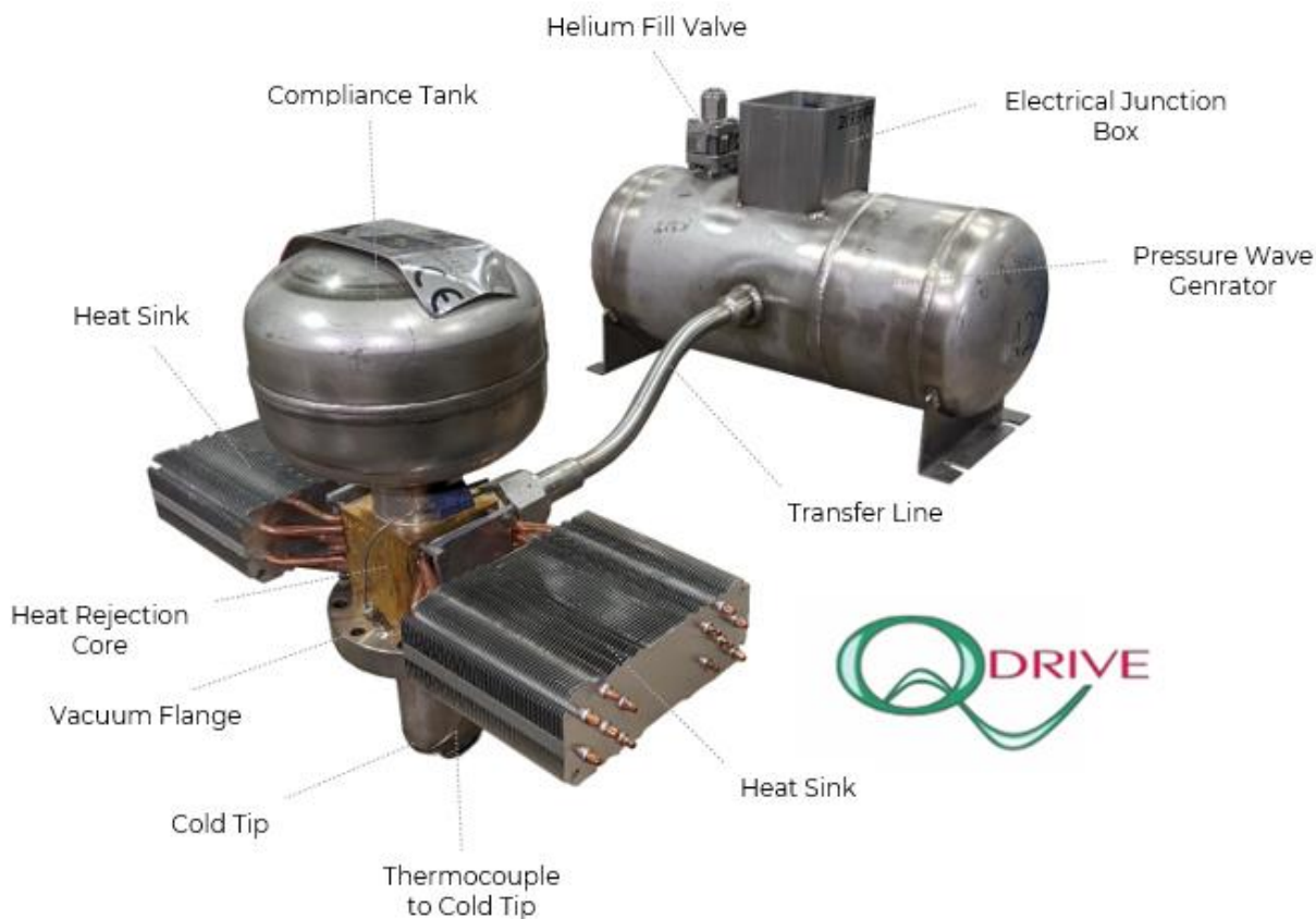
Figure 4: QDRIVE® Cryocooler System
