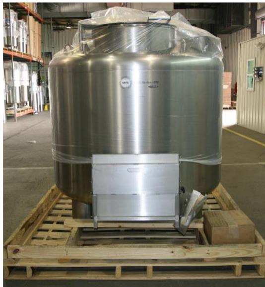
Note: To avoid injury or damaging the equipment, do not apply power to the MVE Variō Pro controller, connect a battery backup, or connect an LN2 supply to the freezer until setup is complete.
