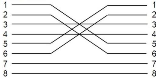
OCAC Master Cable wiring configuration. Numbering as viewed from the side of RJ-45 connector opposite latch.
