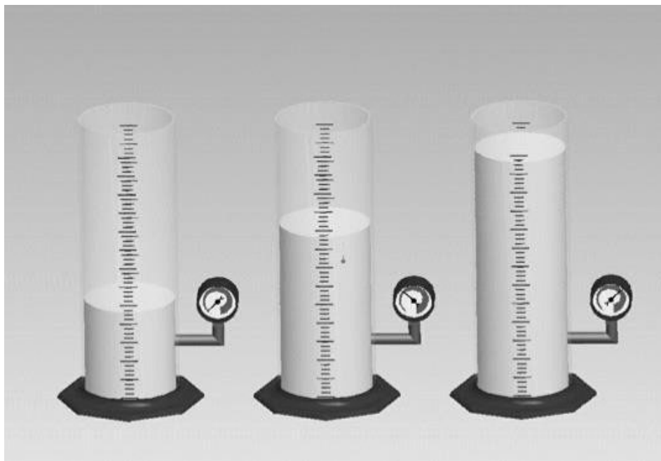
Figure 4: As the fluid level in the cylinder increases, the imposed head pressure at the bottom of the cylinder increases proportionally. The pressure gauges measure this increase in level.
