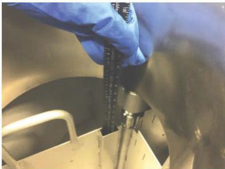
Level dip stick inserted to measure the physical liquid nitrogen level
