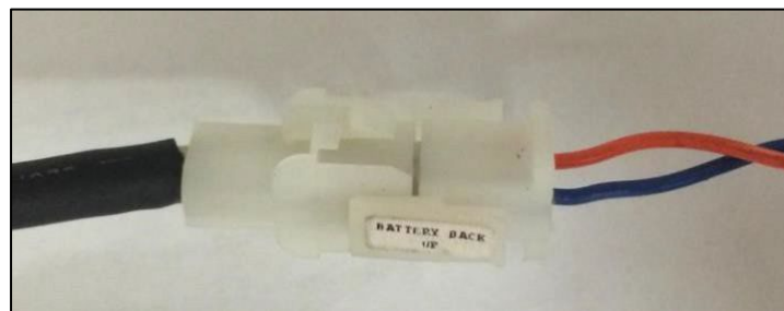
Figure 15 - Battery Backup Connector. [Black – From the Battery Backup. Dark Blue/Orange – From the TEC 3000 Wiring Harness]
